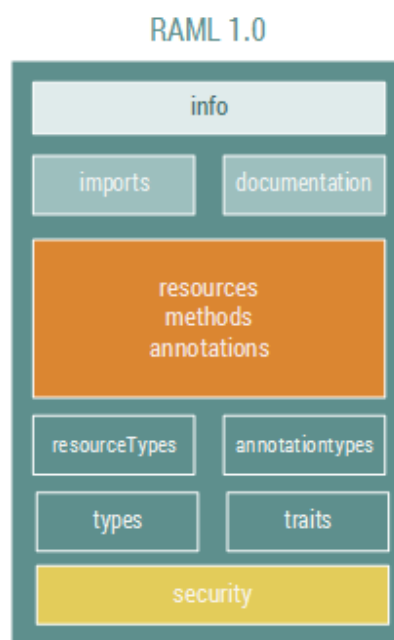
Figure 9: RAML 1.0 general document structure
